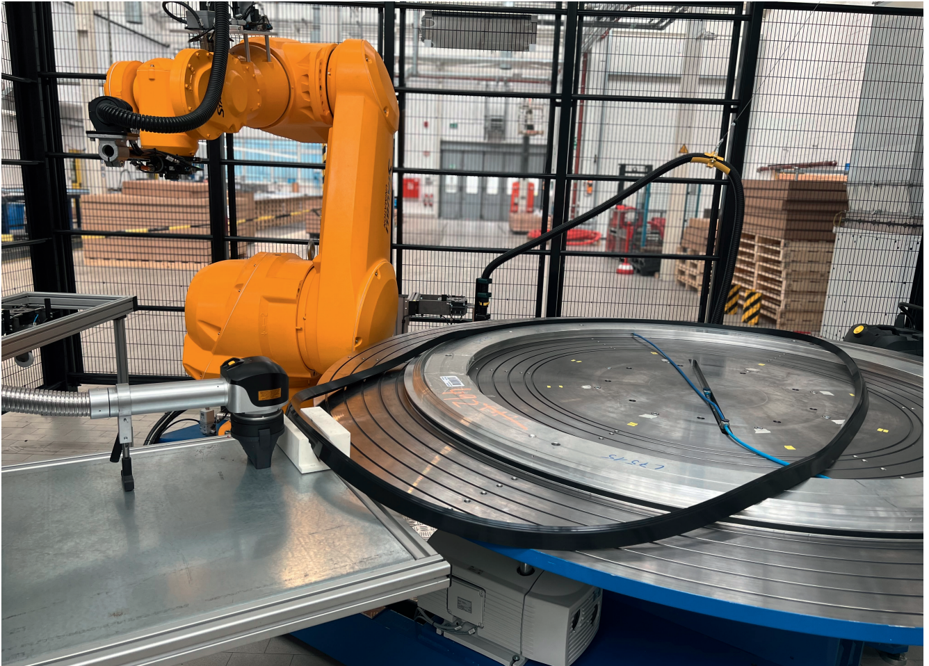
Freudenberg produces customized special seals of up to 12 m in diameter for heavy industry. The engraving laser marks sealing rings clearly, forgery-proof, and permanently to ensure traceability and correct correlation. © Freudenberg Sealing Technologies
