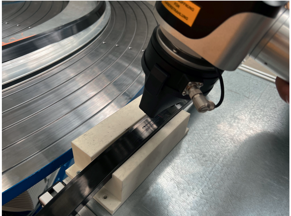
Fig. 2. In a few seconds, the Quasar 20 applies a crisp logo and, for example, the batch or part number. © Freudenberg Sealing Technologies
